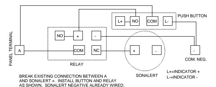
FIG. 5: FIELD INSTALLATION OF SILENCE LATCH
